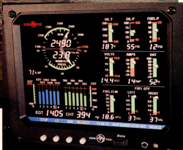
On approach to Albuquerque International Sunport's Runway 3 (above). To enter Albuquerque's airspace from the east, we descended through the pass in the background. JP Instruments' EDM-930 shows the readouts taken when flying at 71 percent power (right).
